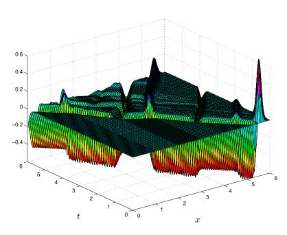
Fig. 8.1. Computation with nonmatching grids on a layered medium with five discontinuities, a pulse created in the surface layer and propagating downward.
