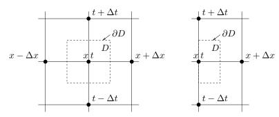
Fig. 5.1. Control volume of an interior grid point and a boundary grid point.
