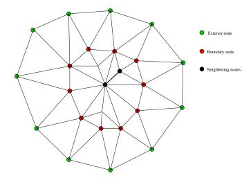
Figure 2: Boundary and exterior nodes in mesh  $\mathcal{T}$
