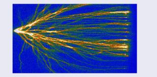
Figure: Positive streamers with a gap of 25 mm shows 70 branches
