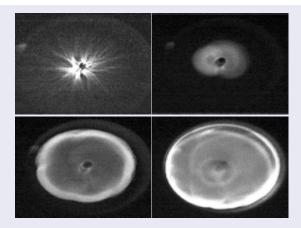
Figure: Sequential photographs (33 ms between images) of axial view of corona discharge ignition of a 6.5% CH4-air mixture at 1 atm, pulse energy 464 mJ, plain electrode. Chamber diameter is 51 mm.
