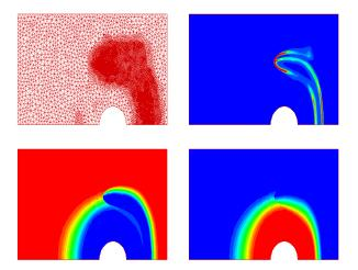
Figure: From left to right and top to bottom: Adaptive mesh, Reaction rate, Oxygen and Fuel
