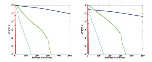
FIG. 5. Convergence curves for the compressible flow: errors in p (on the left) and in u (on the right); GTP-Schur method with no preconditioner (blue), with local preconditioner (green) and with Neumann–Neumann preconditioner (cyan) and GTO-Schwarz method (red).
