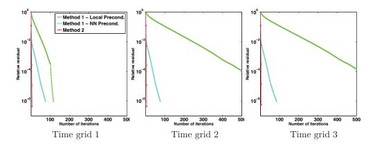
FIG. 7. Relative residual with GMRES for different time grids: GTP-Schur method with the local preconditioner (green), GTP-Schur method with the Neumann–Neumann preconditioner (cyan), and GTO-Schwarz method (red).
