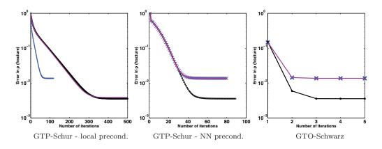
FIG. 9.  $L^2$  pressure error in the fracture: Time grid 1 (blue), Time grid 2 (magenta), Time grid 3 (black).
