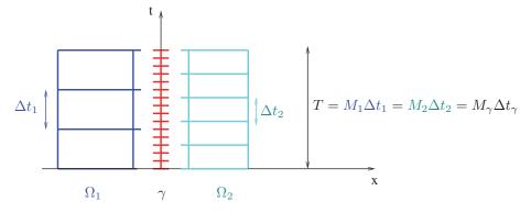
FIG. 2. Nonconforming time grids in the rock matrix and in the fracture.
