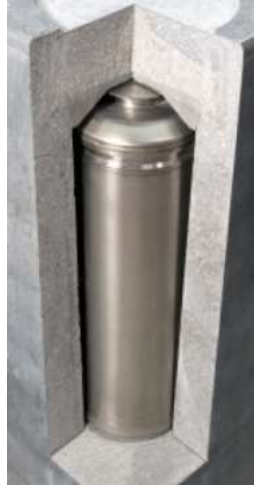
Figure 2: Sealed steel cask of nuclear Waste (Height:1.3m, diameter: 43 cm, approximate weight: 500kg)
