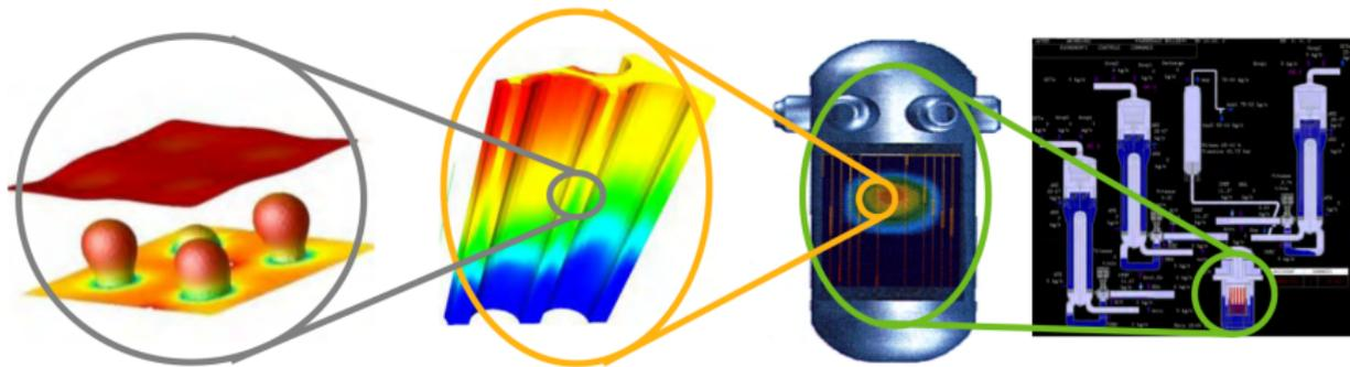
Direct numerical Simulation - Meso-scale - Component scale - System scale
