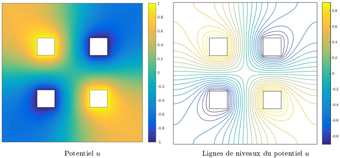
Figure 4.3: Potentiel  $u$  en 2D
