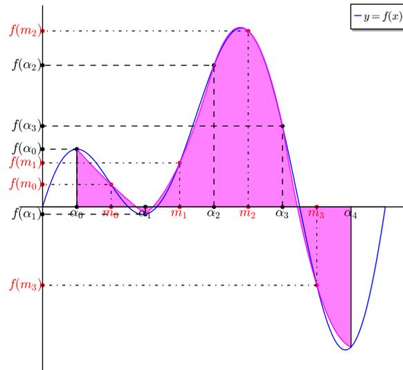
Figure 5.8: Formule composite de Simpson :  $\int_{\alpha}^{\beta} f(x) dx \approx \frac{h}{6} \left( 4 \sum_{j=1}^k f(m_j) + f(\alpha_0) + 2 \sum_{j=1}^{k-1} f(\alpha_j) + f(\alpha_k) \right)$
