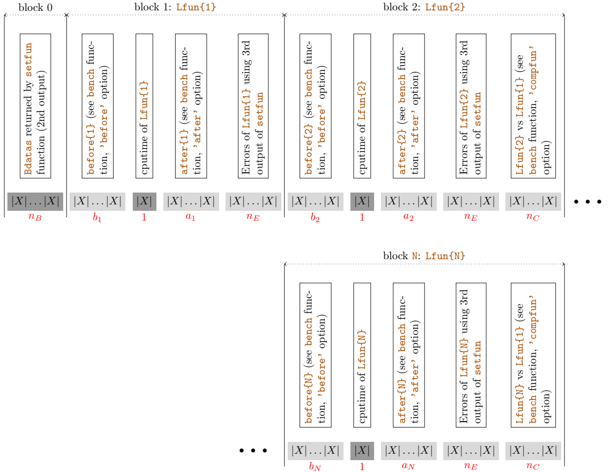
Figure 1: Description of columns of the bench. Each |X| represents one column. Columns with light gray background are optional. Below each subblock (boxes with gray background), the number of columns is given.
