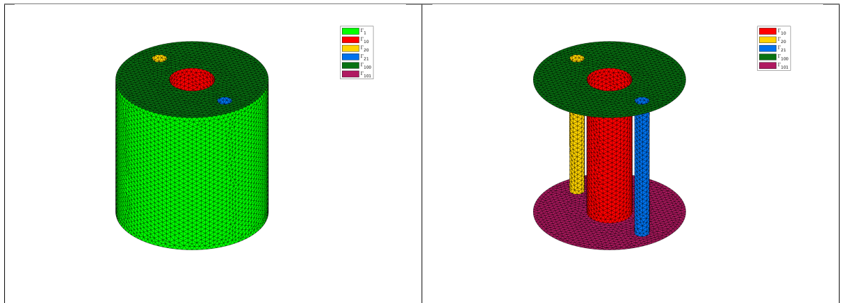
Figure 3.8: 3D stationary convection-diffusion BVP : all boundaries (left) and boundaries without \Gamma_1 (right)
