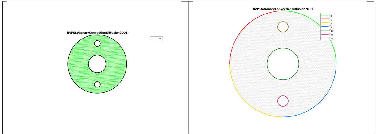
Figure 3.7: 2D stationary convection-diffusion BVP : mesh (left) and boundaries (right)
