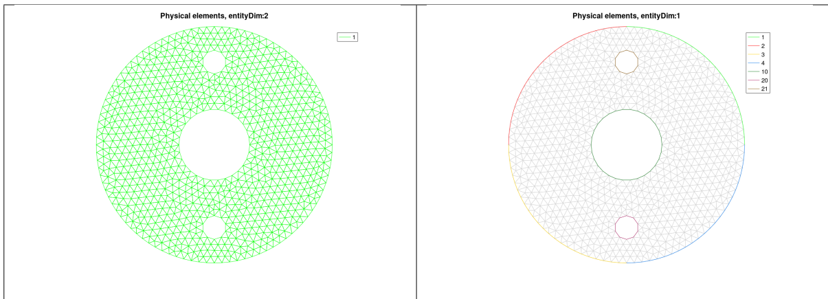
Figure 4: Physical Tag elements of the geofile disk3holes.geo
