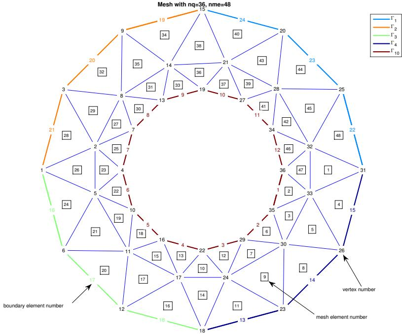
Figure 1: Coarse ring mesh
