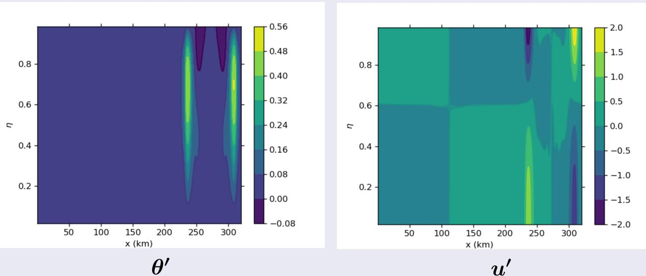
DCMIP 3.1 (Gravity Wave) adapted to slice.  $\Delta x = 1km$ , 30 vertical levels with a Lagrangian vertical coordinate,  $u_0 = 100ms^{-1}$ . 4th-order Runge Kutta time stepping. Shown at t = 1125s. Prognoses  $\Theta$ .
