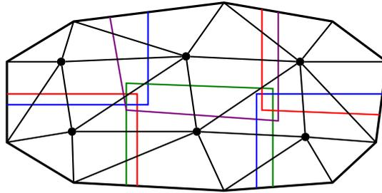
Figure 1: Domain decomposition with a coarse mesh
