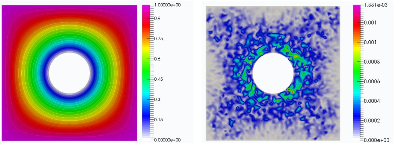
FIGURE 7. Left: solution  $\phi_{\text{map}}$ ; Right: relative error between  $\phi_h$  and  $I_h \phi_{\text{map}}$ .
