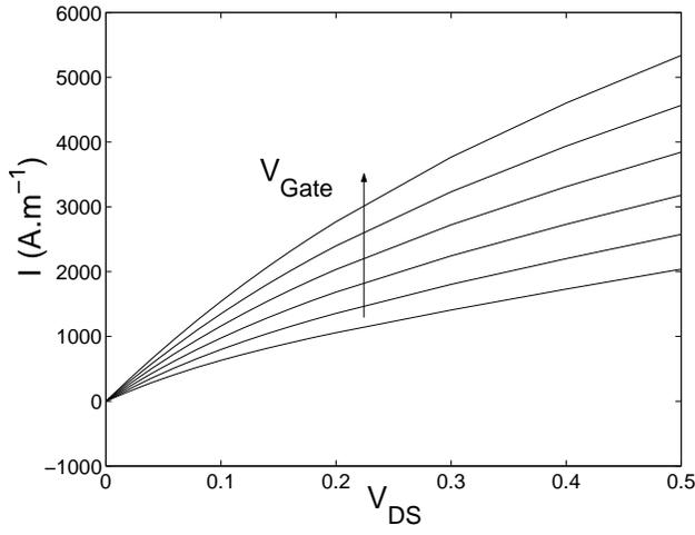
Fig. 2.  $I - V$  characteristics for the device with different gate-source voltage  $V_{GS}$
