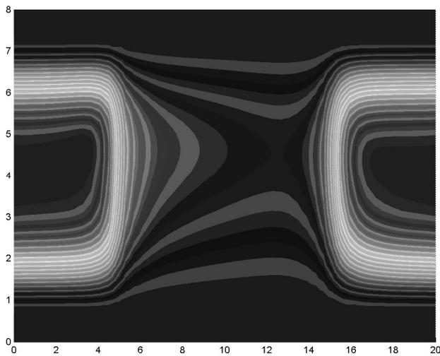
Fig. 6. Density of charge carriers for a applied drain-source voltage  $V_{DS} = 0.2V$  and for  $V_{GS} = 0.2V$
