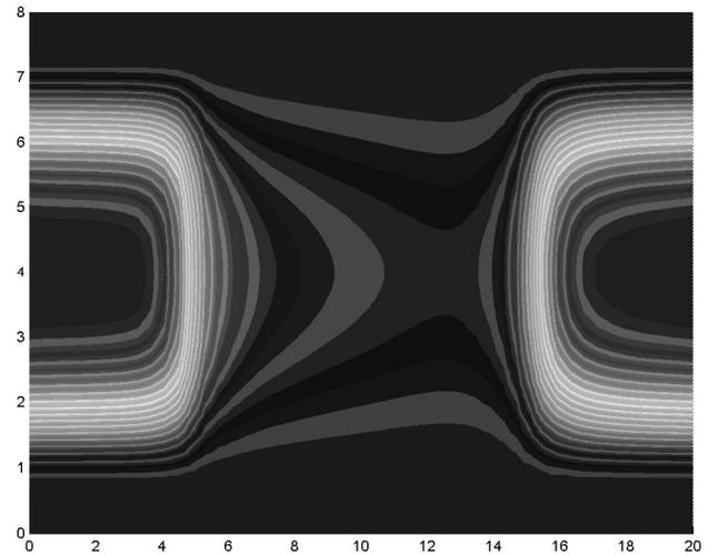
Fig. 5. Density of charge carriers for a applied drain-source voltage  $V_{DS} = 0.2V$  and for  $V_{GS} = 0V$
